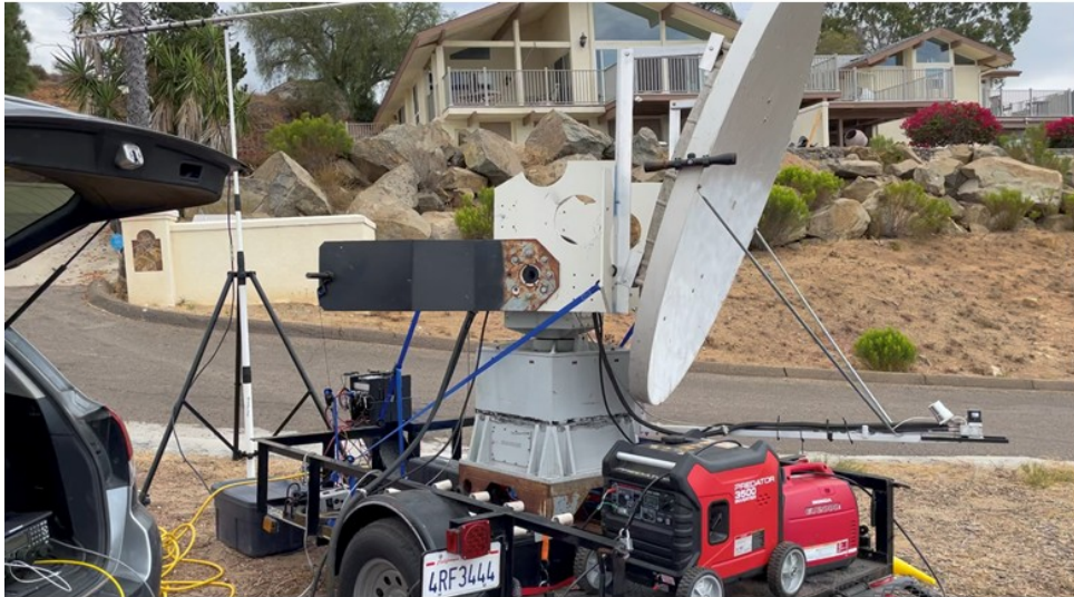
Fig 7: K6MG's portable station with 1.8 metre dish running a TWT at 725 watts; 500 watts to the feed. 432 MHz Yagi for WSPR is at top left of the photo.
